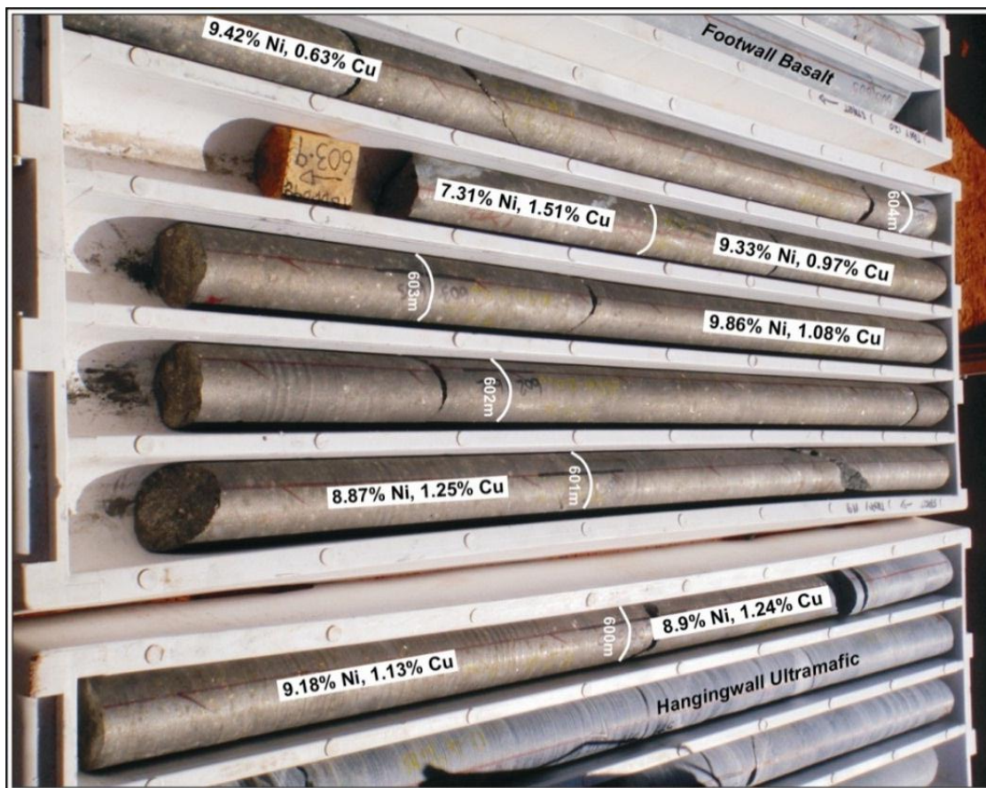
Figure 4: Rosie deposit massive sulphides in TBDD098, with coarse grained pentlandite porphyroblasts.
